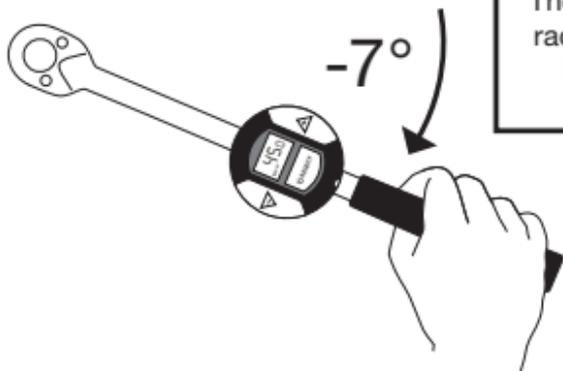
Begin rotating forward again, and press the Select button when resistance is felt. This adds any new movement to the angular rotation saved when ratchet mode was activated.
